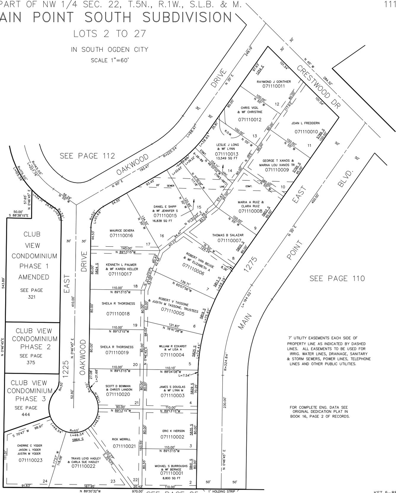
7' UTILITY EASEMENTS EACH SIDE OF PROPERTY LINE AS INDICATED BY DASHED LINES. ALL EASEMENTS TO BE USED FOR IRRIG. WATER LINES, DRAINAGE, SANITARY & STORM SEWERS, POWER LINES, TELEPHONE LINES AND OTHER PUBLIC UTILITIES.
